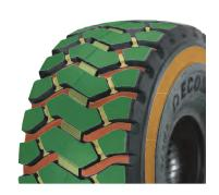
PROTECTED AREA WITH 150% TREAD DEPTH LEVEL GESCHÜTZTE FLÄCHE DURCH 150% PROFILTIEFE
